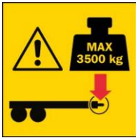
Figure 27. Max. pressure on towing eyelet
