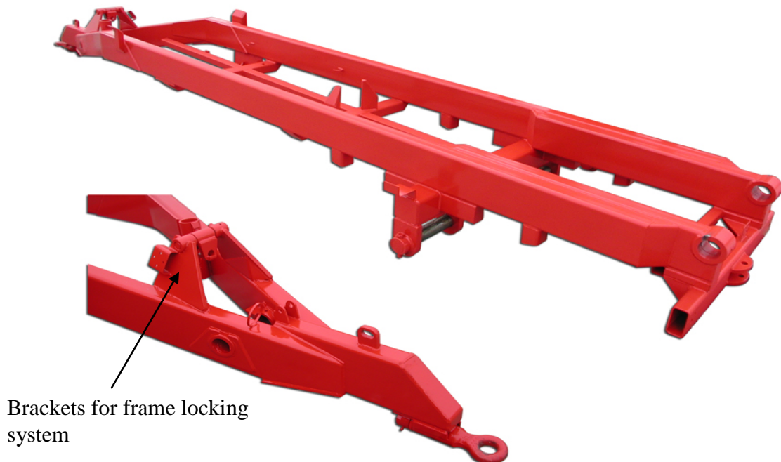
Figure 2b. Chassis with frame locking system
