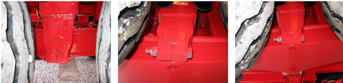
Axel for bogie side Bolts on either side of the bogie Grease nipples
