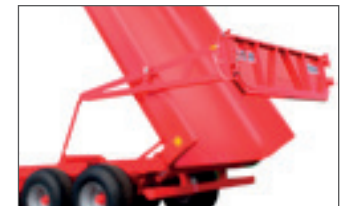
Mechanical lifting tailgate (Only for BT-8)
