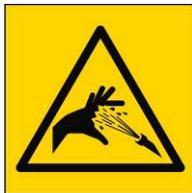
*Figure 22. Hydraulic fluid under pressure*
