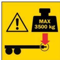
Figure 26. Max. pressure on towing eyelet
