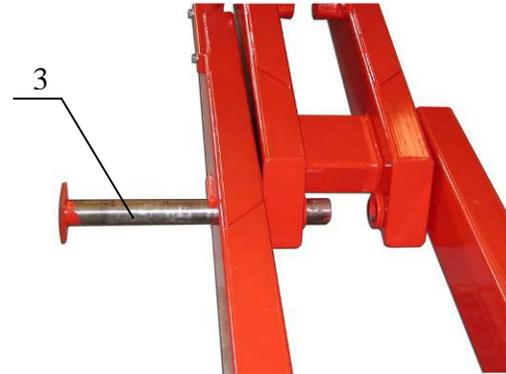
Figure 40. Back and hook frame coupling
