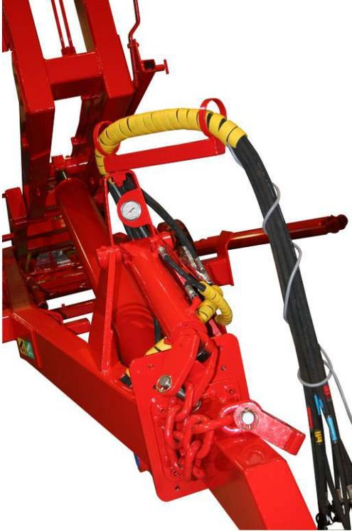
The hydraulic frame lock is used to lock the frame during the exchange function.
