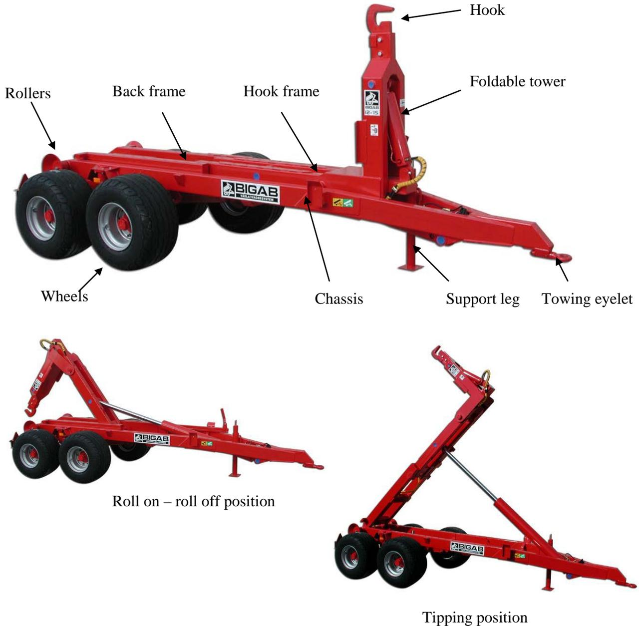
Figure 1. Design of the device
